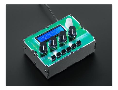
Datadealer is a functionally identical clone of the Mutable Instruments Shruthi-1 - a hybrid analog / digital mono-synth that's as powerful as it is versatile. This thoughtfully curated kit includes all of the components needed to assemble a functioning synthesizer, a lasercut matte black case with iridescent top plate, a set of black Chroma Caps with a glow in the dark encoder cap, and chips pre-loaded with sounds designed and used by Infinity Shred in creating Long Distance.
