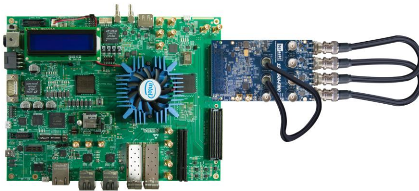
Figure 4-5 Hardware setup of SDI-FMC with A10SoC
