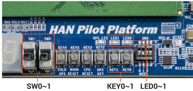
Figure 5-19(5-19) KEYS/SWs/LEDs locations on HAN board
