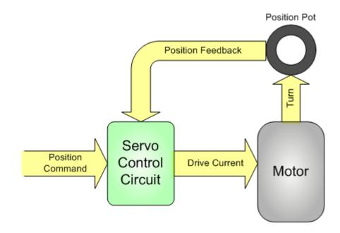
The problem with controlling a standard RC servo motor from a microcontroller is that it is 'closed loop' inside the servo motor case, but 'open loop' with respect to your microcontroller. You can tell the servo control circuit how you want the shaft positioned, but you have no way to confirm if or when this actually happens.
