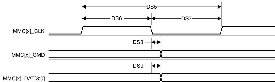
Figure 7-45. MMC – Default Speed – Transmit Mode
