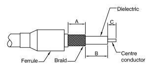
2) Slide the insulator over the dielectric. Crimp the contact onto the centre conductor, using the correct tool.
