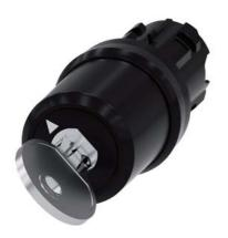
Key-operated switch BKS, 22 mm, round, plastic, lock number S1, with 2 keys, 2 switch positions O-I, latching, actuating angle  $90^\circ$ , 10:30h/13:30h, key removal O, with laser labeling, upper case and lower case, always upper case at the beginning of the word
