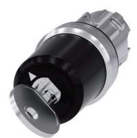
key-operated switch Siemens, 22 mm, round, metal, shiny, lock number SSG10, with 2 keys, 2 switch positions O<I, momentary contact type, actuating angle 45°, 10:30h/12h, key removal O, with laser labeling, upper case and lower case, always upper case at the beginning of the word
