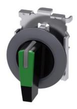
Selector switch, illuminable, 30 mm, round, Metal, matte, green, selector switch, long, front ring for flush installation, 3 switch positions I-O-II, latching, actuating angle 2x45°, 10:30h/12h/13:30h, with laser labeling, inscription or symbol Customer-specific selection with SIRIUS ACT configurator (CIN)
