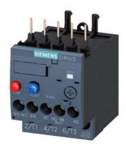
Overload relay 0.18...0.25 A Thermal For motor protection Size S00, Class 10 Contactor mounting Main circuit: Screw Auxiliary circuit: Screw Manual-Automatic-Reset
