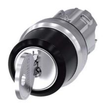
RONIS key-operated switch, 22 mm, round, metal, shiny, lock number SB30, with 2 keys, 3 switch positions I-O-II, latching, actuating angle 2x45°, 10:30h/12h/13:30h, Key removal II, possible special locks: SB31, 421, 455, Z=50-unit packaging
