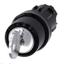
RONIS key-operated switch, 22 mm, round, plastic, lock number SB30, with 2 keys, 3 switch positions I>O<II, momentary contact on the left, latching on the right, actuating angle 2x45°, 10:30h/12h/13:30h, Key removal II, possible special locks: SB31, 421, 455, with laser labeling, upper case and lower case, always upper case at the beginning of the word
