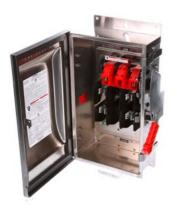
Siemens Low Voltage Circuit Protection Heavy Duty Safety Switches. Type: ENCLOSED, SAFETY SWITCH Std: UL V. Rating: 600V A. Rating: 200A No. Of Poles: 3P F. Rating: 60Hz Action: SINGLE THROW Material: 316SS Enclosure: TYPE 4X. 2-3 point mounting holes. Insulation: YES O. Cycles: 8000 O. Temperature: (-20F-120F) AMBIENT TEMPERATURE Environmental Conditions: INDUSTRIAL CORROSIVE RESISTANCE
