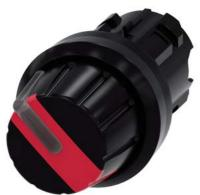
Selector switch, illuminable, 22 mm, round, plastic, red, Rotary knob, 2 switch positions O-I, latching, actuating angle  $90^{\circ}$ , 10:30h/13:30h, with laser labeling, lower case
