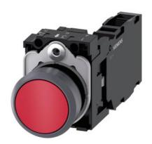
Pushbutton, 22 mm, round, plastic with metal front ring, red, pushbutton, flat, momentary contact type, with holder, 1 NO+1 NC, screw terminal, with laser labeling, upper case and lower case, always upper case at beginning of line
