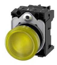
Indicator lights, 22 mm, round, metal, shiny, yellow, lens, smooth, with holder, LED module with integrated LED 24 V AC/DC, screw terminal, with laser labeling, upper case
