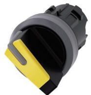
Selector switch, illuminable, 22 mm, round, plastic with metal front ring, yellow, selector switch, short, 2 switch positions O<I, momentary contact type, Actuating angle 45°, 10:30h/12h, with laser labeling, upper case
