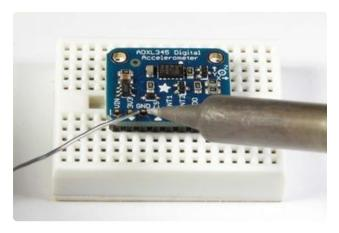
And Solder Be sure to solder all pins to assure good electrical contact.
