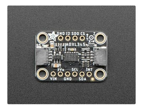
The sensor has three axes of measurements, X Y Z, and pins that can be used either as I2C or SPI digital interfacing. You can set the sensitivity level to either +-2g, +-4g, +-8g or +-16g. The lower range gives more resolution for slow movements, the higher range is good for high speed tracking. The ADXL345 is the latest and greatest from Analog Devices, known for their exceptional quality MEMS devices.
