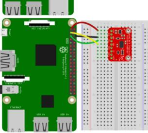
Connect SCL (yellow wire in STEMMA QT version) on the RPi to SCL on the ADXL343 Connect SDA (blue wire in STEMMA QT version) on the Rpi to SDA in the ADXL343 Connect GND (black wire in STEMMA QT version) on the Rpi to GND on the ADXL343
