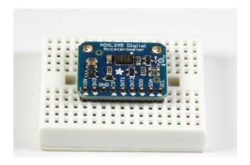
Add the Breakout Align the breakout board and place it over the header pins on the breadboard.
