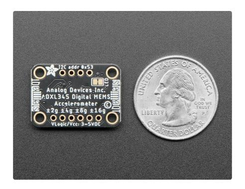
We added an on-board 3.3V regulator and logic-level shifting circuitry, making it a perfect choice for interfacing with any 3V or 5V microcontroller or computer, such as Arduino or Raspberry Pi.
