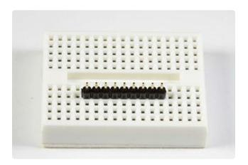
Position the Header Cut the header to size if necessary. Then plug the header - long pins down - into a breadboard to stabilize it for soldering.
