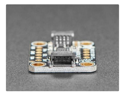
As if that weren't enough, we've also added <u>SparkFun qwiic</u> () compatible <u>STEMMA</u> QT () connectors for the I2C bus so you don't even need to solder. Just wire up to
