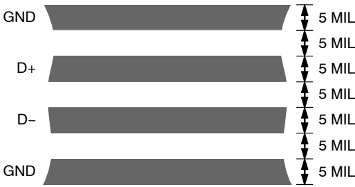
Figure 21. Typical Arrangement of Signal Tracks
