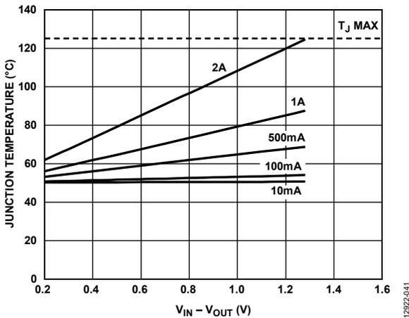
Figure 41. 500 mm<sup>2</sup> of PCB Copper,  $T_B = 50^\circ\text{C}$
