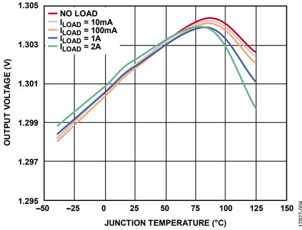
Figure 4. Output Voltage ( $V_{OUT}$ ) vs. Junction Temperature
