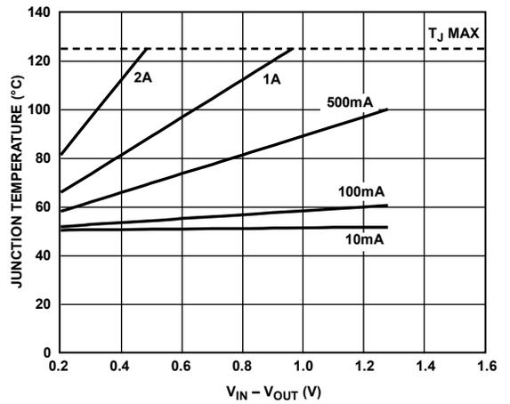
Figure 38. 500 mm<sup>2</sup> of PCB Copper,  $T_A = 50^\circ\text{C}$
