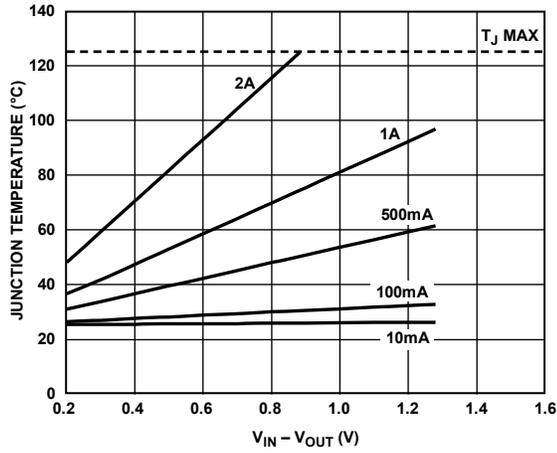
Figure 34. 6400 mm<sup>2</sup> of PCB Copper,  $T_A = 25^\circ\text{C}$
