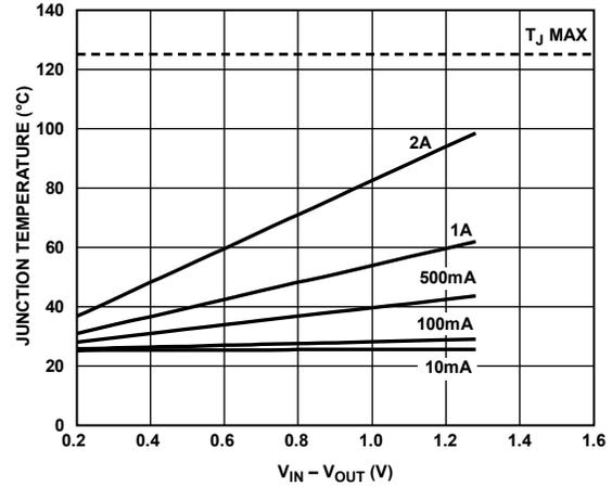
Figure 42. 1000 mm<sup>2</sup> of PCB Copper,  $T_B = 25^\circ\text{C}$
