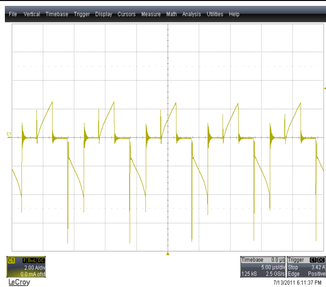
Figure 25 - Primary current with programmed imbalance between PWMs (less than 180µs), 8A load
