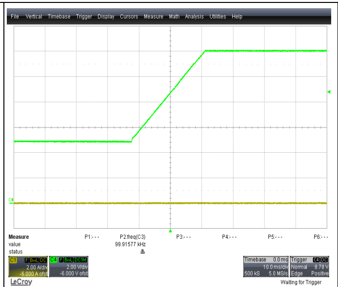
Figure 15 - Startup with softstart from pre-charge Green trace: Output voltage Yellow trace: Output load current
