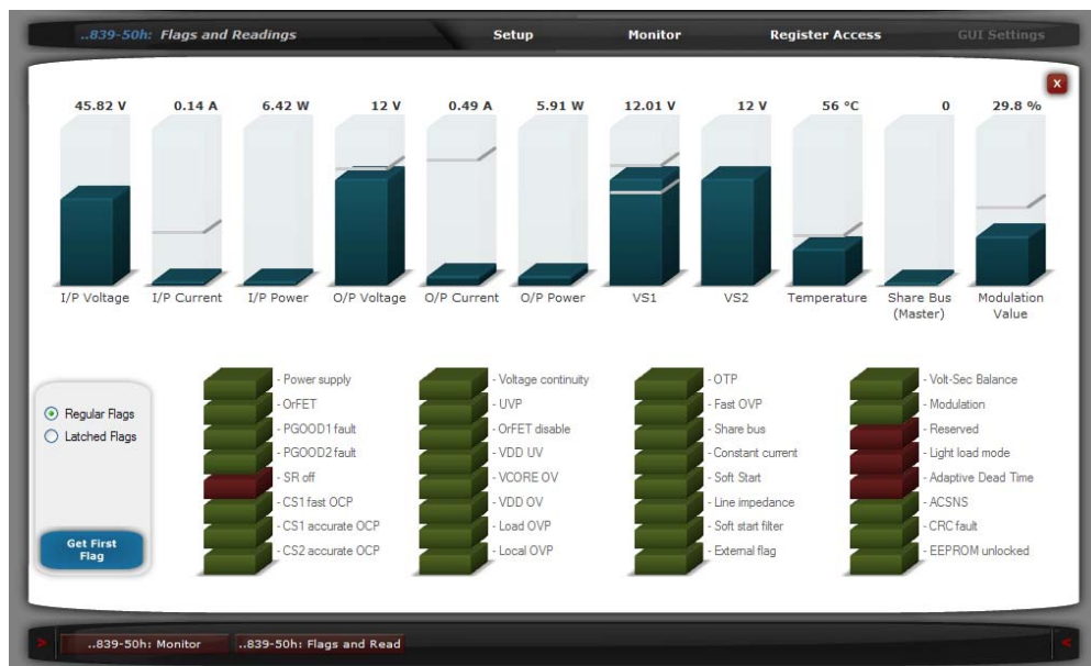
Figure 33 - ACSNS flag tripped during light load mode
