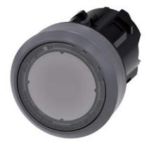
Pushbutton, 22 mm, round, plastic with metal front ring, clear, pushbutton, flat momentary contact type, with laser labeling, inscription or symbol Customer-specific selection with SIRIUS ACT configurator (CIN)
