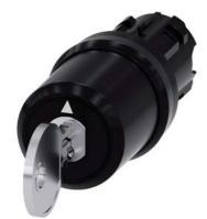
key-operated switch Siemens, 22 mm, round, plastic, lock number SSG10, with 2 keys, 3 switch positions I-O<II, left latching, momentary contact type on the right, actuating angle 2x45°, 10:30h/12h/13:30h, key removal O+I, with laser labeling, upper case and lower case, always upper case at beginning of line
