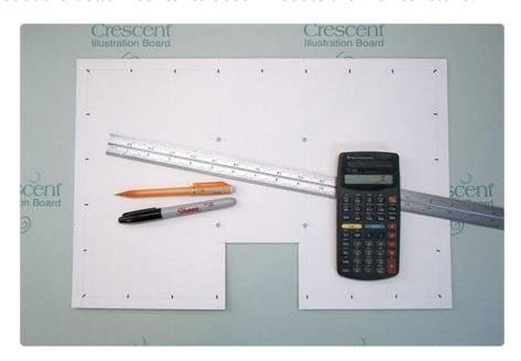
Next, calculate the spacing for a ring of 25 LEDs. For this monitor, it worked out nicely as a 9x6 rectangle, roughly 2" spacing, with a one pixel gap at the bottom where the monitor stand protrudes. Perfect!
