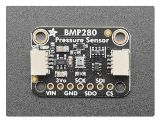
Adafruit BMP280 I2C or SPI Barometric Pressure & Altitude Sensor
