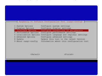
Run sudo raspi-config to configure the system, and select Interfacing Options.
