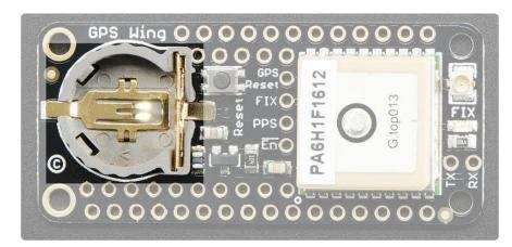
The GPS does not require but does benefit by having a coin cell backup battery. You can install any "CR1220" sized battery into the holder. The GPS will automatically detect the battery and use it as a backup for the ephemeris memory
