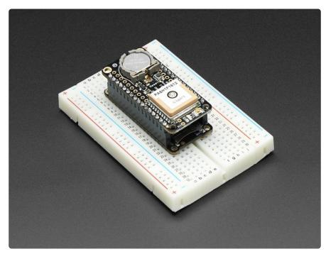
The GPS has a built in real time clock, which can keep track of time even when it power is lost and it doesn't have a fix yet. It can also help reduce fix times, if you expect to have a flakey power connection (say you're using solar or similar). To use the RTC, we need to install a battery. We provide the holder but the battery is not included. You can use any 12mm coin cell - these are popular and we also carry them in the Adafruit shop.
