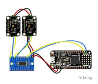
Board 3V to mux VIN (red wire)
