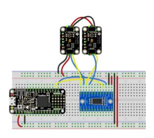
Board 3V to mux VIN (red wire)
