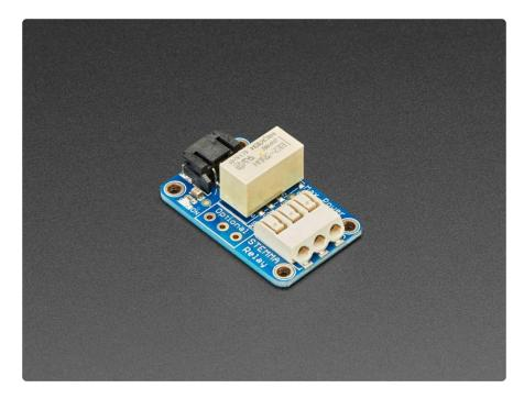
Each STEMMA board comes with a fully assembled and tested PCB but no cable. No soldering is required to use it. There's an optional second switch on the side of the PCB, if you get a 3-pin terminal block () you can solder that in place, but its optional.
