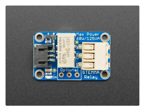
No worrying about flyback diodes, level shifting, pin protection. The STEMMA board takes care of all that for you. You can use it with any 3V or 5V microcontroller/ microcomputer. To use with a breadboard, Raspberry Pi or Arduino (), pair with a JST
