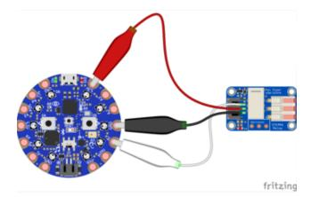
Plug the 3-pin JST to alligator clip cable into the 3-pin JST connector on the STEMMA Relay Connect the white alligator clip to A1 Connect the black alligator clip to GND Connect the red alligator clip to 3.3v
