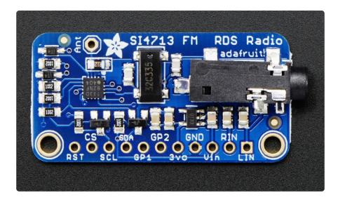
Yaaar! Become your very own pirate radio station with this FM radio transmitter. This breakout board, based on the best-of-class Si4713, is an all-in-one stereo audio FM transmitter that can also transmit RDS/RBDS data!
