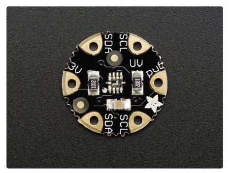
The Si1145 is an I2C sensor, so there are not a lot of pins to worry about.
