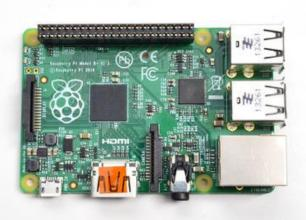
Start by plugging the 2x20 header into a Raspberry Pi, this will keep the header stable while you solder. Make sure the Pi is powered off!
