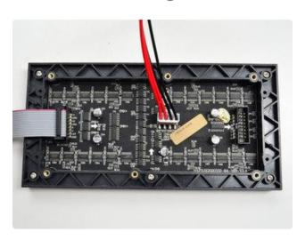
IDC goes into the INPUT side (look for any arrows, arrows point from INPUT side to OUTPUT)
