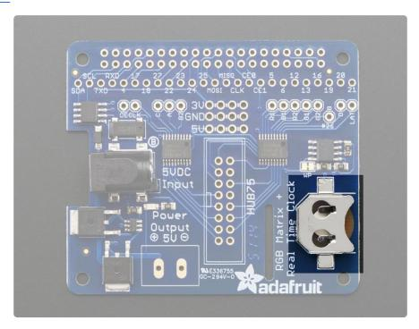
The **rgb-matrix.sh** script already installed the necessary software to use the realtime clock...but you'll need to set the initial time once. This is explained in the <u>"Sy</u> nc time from Pi to RTC" section of this DS1307 tutorial () (just that one section...you can ignore the rest).
