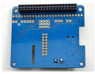
Flip the board over, the tape should keep the connector from falling out
