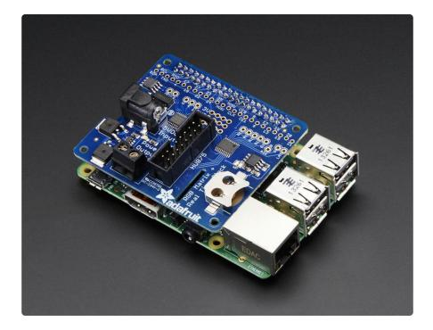
Works with any of our <u>16x32</u>, <u>32x32</u> or <u>32x64</u> RGB LED Matrices with HUB75 connections (). The latest "Rev C" HAT also supports 64x64 matrices by soldering a small jumper on the PCB. You can even chain multiple matrices together for a longer display - we've only tested up to 32x128 but it works just fine. The bigger the display the harder it is on the Pi, so keep that in mind if you're using a lower-powered Pi Zero.
