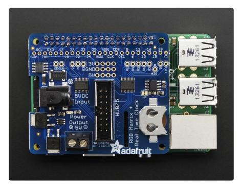
Each order comes with a HAT PCB with all surface mount parts assembled, a 2x20 female socket connector, a 2 pin terminal block, and a 2x8 IDC socket connector. A
