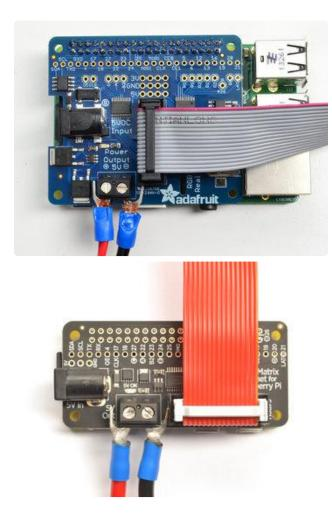
The RGB matrix also came with a 2x8 data cable. Connect one end to the matrix's INPUT side and the other end to the IDC socket on the HAT/bonnet.
