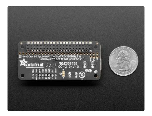
Works with any of our 16x32, 32x32 or 32x64 RGB LED Matrices with HUB75 connections (). You can also use 64x64 matrices by soldering a small jumper on the PCB (). Want more lights? No problem, chain multiple matrices together for a longer display - we've only tested up to 32x128 but it works just fine. The bigger the display the harder it is on the Pi, so keep that in mind if you're using a lower-powered Pi Zero.
