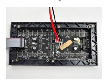
IDC goes into the INPUT side (look for any arrows, arrows point from INPUT side to OUTPUT)
