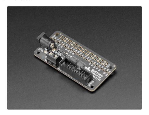
"Bonnet" boards work on any Raspberry Pi with a 40-pin GPIO header — Zero, Zero W/WH, Model A+, B+, Pi 2, 3 and 4. They do not work with older 26-pin boards like the original Model A or B. Note with the Pi Zero you may need to solder a header on the Pi board; it's normally unpopulated on that model (except the "Zero WH").
