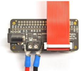
The RGB matrix also came with a 2x8 data cable. Connect one end to the matrix's INPUT side and the other end to the IDC socket on the HAT/bonnet.
