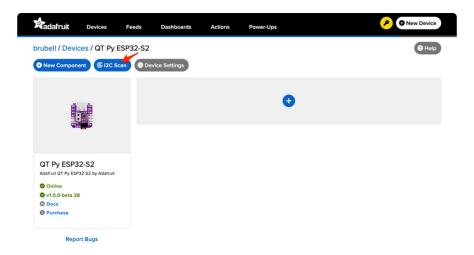
You should see a new pop-up showing a list of the I2C addresses detected by an I2C scan. If wired correctly, the AHT20's default I2C address of 0x38 appear in the I2C scan list.
