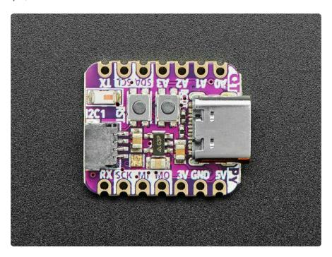
The ESP32-S2 is a highly-integrated, low-power, 2.4 GHz Wi-Fi System-on-Chip (SoC) solution that now has built-in native USB as well as some other interesting new technologies like Time of Flight distance measurements. With its state-of-the-art
