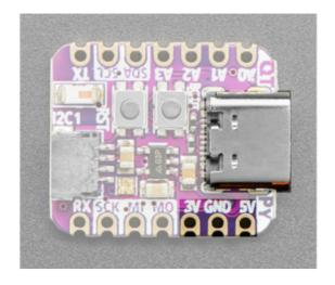
USB-C port - This is used for both powering and programming the board. You can power it with any USB C cable.
