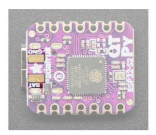
BAT/GND pads - On the back of the board are two pads labeled BAT and GND. These are the battery input pads with diode protection for external battery packs from 3V to 6V input.
