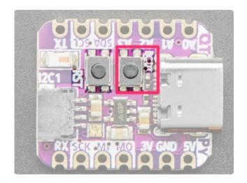
Your QT Py has two buttons: a reset button and a boot button. This page will use the boot button (highlighted in pink), located underneath the QT Py's USB-C cable.
