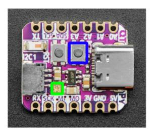
The RGB NeoPixel LED (highlighted in green) is located near the SCK/MI on the board silk, at the corner of the STEMMA QT sensor.
