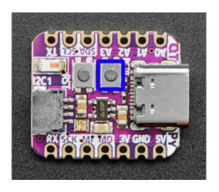
The boot button (highlighted in blue) is labeled Boot on the silk, and is located at the corner of the USB connector.
