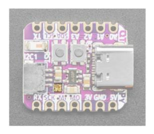
Above the SCK and MI on the silk, is the RGB NeoPixel LED. This addressable LED works both as a status LED (in CircuitPython and the bootloader), and can be controlled with code. It is available in CircuitPython as board.NEOPIXEL, and in Arduino as PIN NEOPIXEL.
