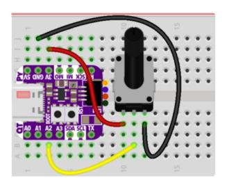
QT Py 3V to potentiometer left pin QT Py A2 to potentiometer middle pin QT Py GND to potentiometer right pin
