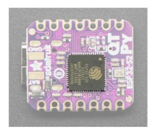
The ESP32-S2 is a highly-integrated, low-power, 2.4 GHz Wi-Fi System-on-Chip (SoC) solution that now has built-in native USB as well as some other interesting new technologies like Time of Flight distance measurements. With its state-of-the-art power and RF performance, this SoC is an ideal choice for a wide variety of application scenarios relating to the Internet of Things (IoT) (), wearable electronics (), and smart homes.
