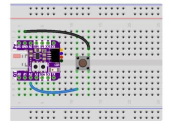
Make the following connections between the QT-PY and the button:
