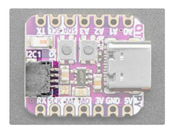
The QT Py ESP32-S2 has TWO I2C ports!
