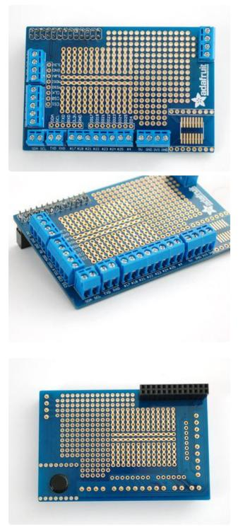
Place the blue terminal blocks around the perimeter of the Proto Plate PCB. Make sure you place them so that the open ends are facing out as shown.
