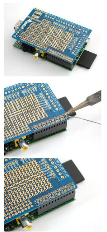
Place the proto plate PCB on so that the 2x13 header pins poke out through the matching 2x13 pads in the corner.
