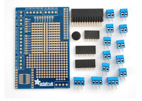
The layout of the board is a mix between 'breadboard style' (top middle) - with two 'rails' down the center and then 5-pin connected rows along-side. This layout is familiar for anyone who has used a breadboard. The remaining holes are 'perf' style no connection between them. This allows for more flexibility.
