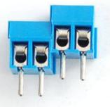
Find the terminal blocks, they're blue and come in 3-pin and 2-pin shapes. We'll need to slide the blocks together for the next step where we put the blocks into the proto plate. Slide them together to make 1x8 pin, 1x5 pin, and 3x4pin terminal blocks
