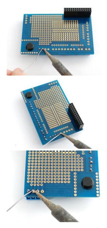
Solder each terminal block connection to the PCB using plenty of solder to make a strong mechanical connection
