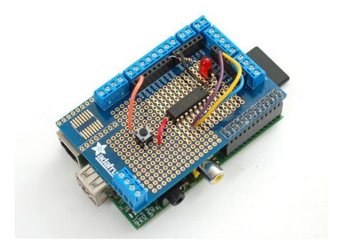
The terminal blocks make it easy to connect to wires for installations. Simply use a small Philips or flathead to open up the block, insert a stranded or solid core wire, then tighten it down.
