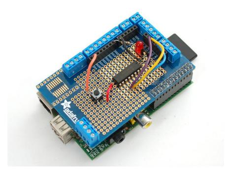
Now that you've finally got your hands on a <u>Raspberry Pi</u><sup>®</sup> (), you're probably itching to make some fun embedded computer projects with it. What you need is an add on prototyping Pi Plate from Adafruit, which can snap onto the Pi main board assembly (and is removable later if you wish) and gives you all sorts of prototyping goodness to make building on top of the Pi super easy.
