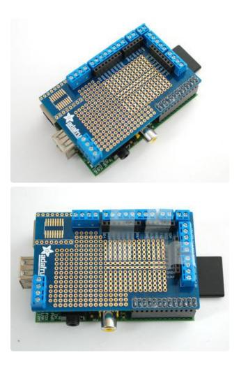
This part is optional, but if you want to have sockets for the GPIO pins so you can plug wires in and out easily, you can solder in the two 8-pin and single 6-pin header.
