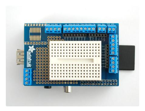
We designed the plates so you can fit a 'tiny breadboard' (http://adafru.it/65) on top and still see the pin labels on the breakouts. This makes it easy to do fast prototyping!
