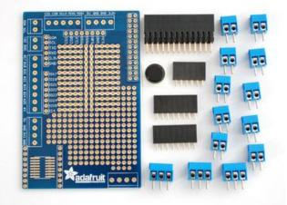
Check that you have all the parts - a PCB, a 2x13 female header, a 1x6 female header, two 1x8 female headers, bumper, three 3pin terminal blocks and ten 2-pin terminal blocks
