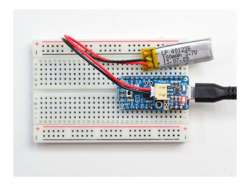
If you want to add an On/Off switch, we also made that really easy. The two 0.1" holes with a box around them are the battery output line. Carefully cut the trace between them with a hobby knife and replace with two wires from a switch like this slide switch (), or this pushbutton one (http://adafru.it/1683), for example.
