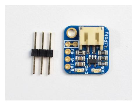
Solder the backpack on with the extra long header so that it can still plug into a breadboard, or clip the long header leads short afterwards for a slim package.
