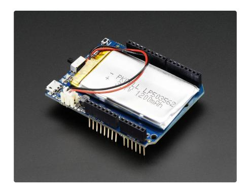
The PowerBoost shield can run off of any Lithium Ion or Lithium Polymer battery (3.7/4.2V kind) but we suggest our 1200mAh capacity one which fits very nicely in the empty space of the shield. Plug in the battery and recharge it via the microUSB jack. When you're ready to go, just unplug the Arduino from USB or the wall adapter and it will automatically switch over to shield power.
