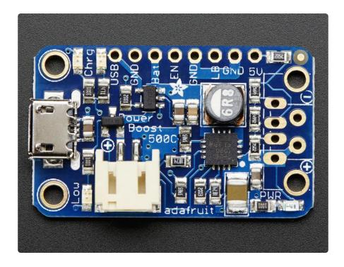
The PowerBoost 500C has at the heart a <u>TPS61090 boost converter from TI</u> (). This boost converter chip has some really nice extras such as low battery detection, 2A internal switch, synchronous conversion, excellent efficiency, and 700KHz high-frequency operation. Check out these specs!
