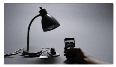
A Feather board without ambition is a Feather board without FeatherWings! This is the Power Relay FeatherWing. It gives you power to control, and control over power. Put simply, you can now turn on and off lamps, fans, solenoids, and other small appliances that run on up to 250VAC or DC power using any Feather board. <u>Compare</u> d to our smaller mini Relay FeatherWings (), this one can handle a beefy 1200 Watts!
