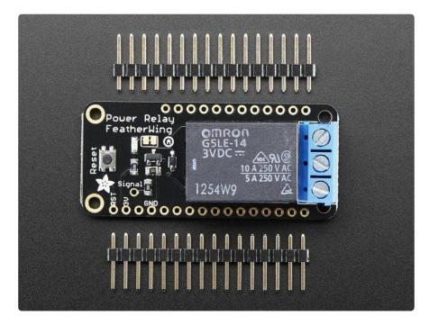
Each FeatherWing comes with a fully assembled and tested PCB, header you can use to attach to your Feather. By soldering closed the jumper on the underside of the Wing you can select which pin you want to use for the relay control. Some light soldering is required.
