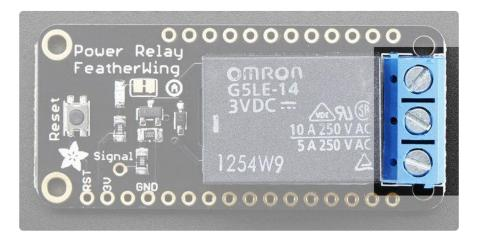
The Wing has the power control output on the end, a 3-pin 5.08 mm terminal block. The COM pin is what you should connect the signal you're planning to switch.
