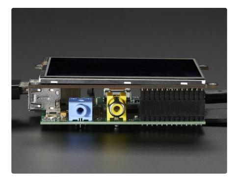
Uses the hardware SPI pins (SCK, MOSI, MISO, CE0, CE1) as well as GPIO #25 and #24. GPIO #18 can be used to PWM dim the backlight if you like. All other GPIO are unused. There's a 2x13 header on the bottom, you can connect a standard Pi GPIO cable to it to use any of the other pins ask you like
