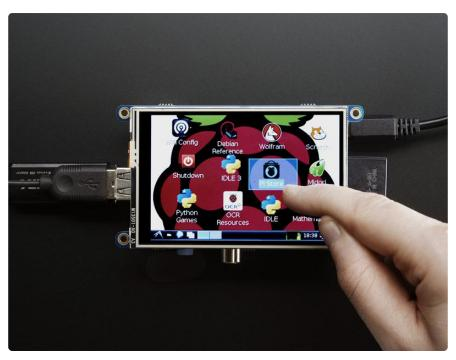
Is this not the cutest, little display for the Raspberry Pi? It features a 3.5" display with 480x320 16-bit color pixels and a resistive touch overlay, but is only slightly larger than <u>our popular original</u> (). The plate uses the high speed SPI interface on the Pi and can use the mini display as a console, X window port, displaying images or video etc. Best of all it plugs right in on top!
