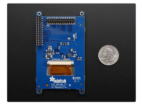
Best of all, it comes fully assembled and ready to plug into your Pi! You can use this as a display for running the X interface, or pygame. You can also have an HDMI display seperately connected.
