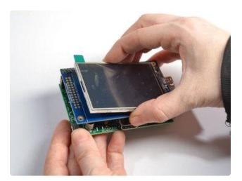
Line up the screen on the white outline, make sure there's some space from the header you just soldered in and the metal sides of the screen. As long as you don't really press down on the screen you can reposition it once or twice.
