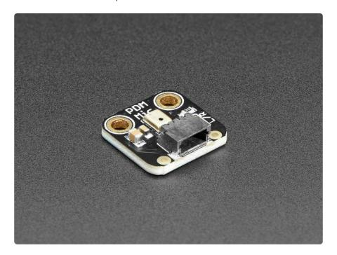
The first thing to note is that this sensor does not provide an 'analog' output like many of our electret microphone assemblies. So it's great for chips that do not have analog inputs. Secondly, the digital interface is a very simplistic pulse density modulation
