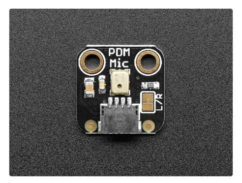
The 4-pin JST connector has 3V, GND, DAT, CLK connections that <u>can be used with</u> <u>one of our JST-SH cables to make a flexible mic arrangement</u> (). <u>If you want a version</u> <u>with breakout headers, we have a version here</u> (). An on-board solder jumper lets you change the mic from Left to Right channel
