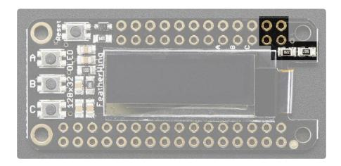
The cute little OLED does all of the data transfer over the I2C pins, highlighed above SDA and SCL. No other pins are required. There are two 2.2K pullups to 3V on each.
