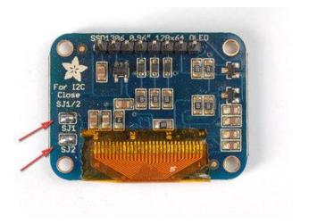
Microcontroller 3V to OLED Vin Microcontroller GND to OLED Gnd Microcontroller SCL to OLED Clk Microcontroller SDA to OLED Data Microcontroller D9 to OLED Rst
