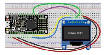
Microcontroller 3V to OLED Vin
