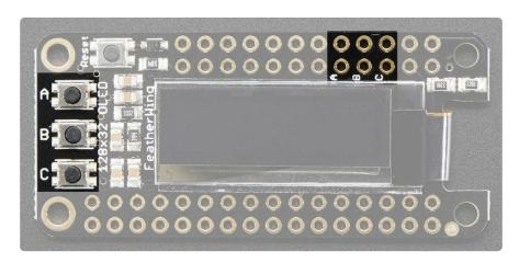
We had a little bit of space so we added three mini tactile buttons that you can use for user interface. We label them A B and C because each Feather has slightly different pin numbering schemes and we wanted to make it 'universal'
