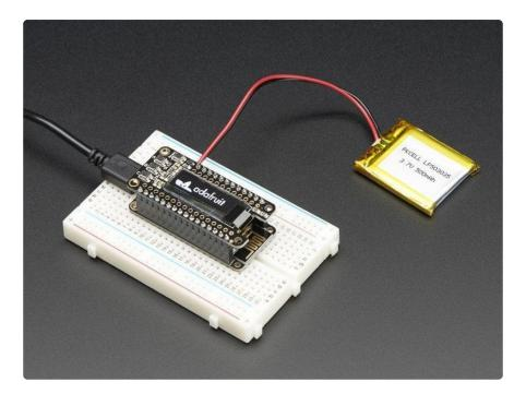
A Feather board without ambition is a Feather board without FeatherWings! This is the FeatherWing OLED: it adds a 128x32 monochrome OLED plus 3 user buttons to an y Feather main board. Using our <u>Feather Stacking Headers</u> (http://adafru.it/2830) or <u>Feather Female Headers</u> (http://adafru.it/2886) you can connect a FeatherWing on top of your Feather board and let the board take flight!
