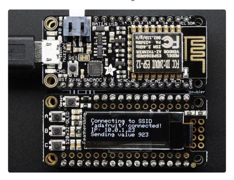
These displays are small, only about 1" diagonal, but very readable due to the high contrast of an OLED display. This screen is made of 128x32 individual white OLED pixels and because the display makes its own light, no backlight is required. This
