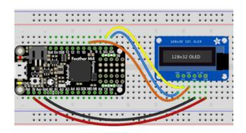
Microcontroller 3V to OLED VIN
