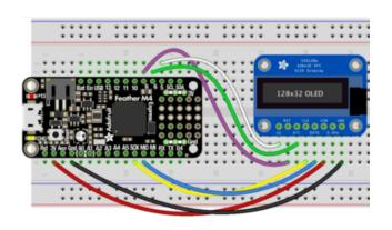
Microcontroller 3V to OLED VIN
