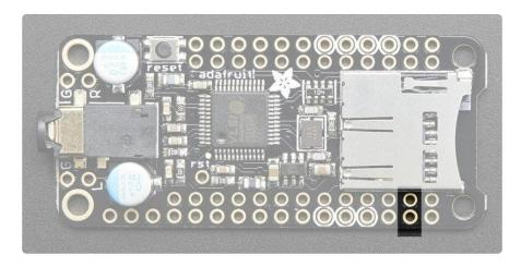
This is the UART data pin that is connected to the MIDI RX on the VS1053. If you short the jumper on the back to put it in MIDI mode, you can send data from the TX pin.
