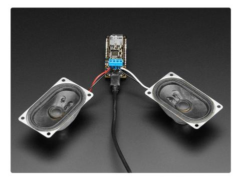
All this functionality is implemented in a light-weight SPI interface so that any Feather Board can play audio from an SD card. There's also a special MIDI mode that you can boot the chip into that will read 'classic' 31250Kbaud MIDI data from the UART TX pin and act like a synth/drum machine - there are dozens of built-in drum and sample effects!
