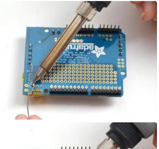
Then flip the board over and solder the 6 pins
