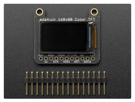
The board comes with all surface-mount components pre-soldered. The included header strip can be soldered on for convenient use on a breadboard or with 0.1" connectors. You can also skip this step and solder on wires.
