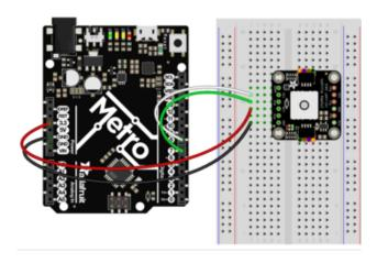
3.3 to VIN GND to GND 8 to TXO 7 to RXI
