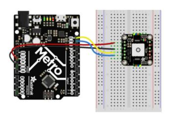
VIN to 3.3 GND to GND SDA to SDA SCL to SCL
