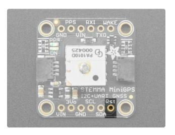
RST - When pulled to ground, this will put the chip in the module into reset. Handy when you want to start with a completely clean setup.
