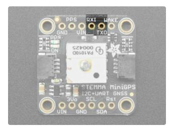
TXO - the pin that transmits data from the GPS module to your microcontroller or computer. It is 3.3V logic level. Data comes out at 9600 baud 8N1 by default RXI - the pin that you can use to send data to the GPS. This pin is level shifted so you can use 3-5V logic. By default it expects 9600 baud data by default.
