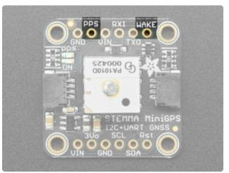
PPS is a "pulse per second" output. Most of the time it is at logic low (ground) and then it pulses high (3.3V) once a second, for 50-100ms, so it should be easy for a microcontroller to sync up to it WAKE - This pin works with low power and standby modes. Check the datasheet for more information!
