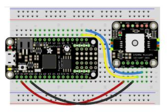
Feather 3V to module VIN Feather GND to module GND Feather SCL to module SCL Feather SDA to module SDA
