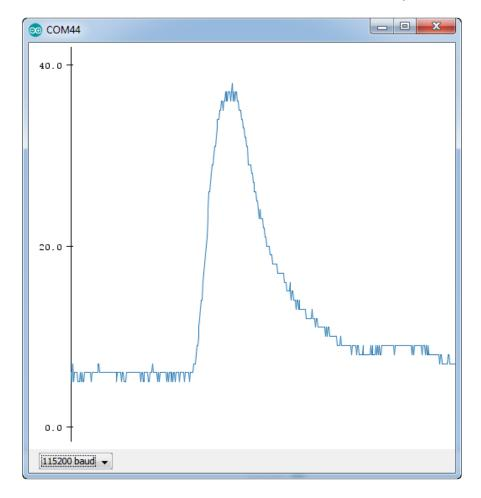
Note that the sensor is sensitive to multiple gasses - but cannot tell which it is! That's normal, most gas sensors are like that - so it is best for measuring changes in a know n gas density, not detecting which is changing.
