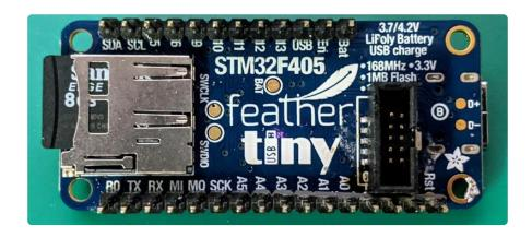
The Feather STM32F405 Express uses SDIO to connect its built in micro SD card slot. Didn't notice it had an SD card slot? We hid it on the underside.
