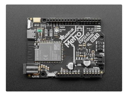
What's Metro shaped and has an ESP32-S2 WiFi module? What has a STEMMA QT connector for I2C devices, and a Lipoly charger circuit? That's right - its the Adafruit Metro ESP32-S2!
