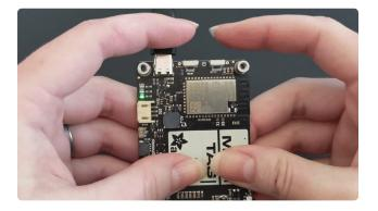
For all ESP32-family boards, you can enter the ROM bootloader by holding down the BOOT button while clicking RST.
