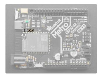
The hardware UART debug port has two broken out pins. You can connect these to a USB console cable in order to read the debug output from the ESP32 IDF (). This is useful if you are writing software and need to see the low level debug output without using JTAG debugging.
