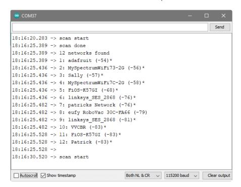
If you can not scan any networks, check your power supply. You need a solid power supply in order for the ESP32 to not brown out. A skinny USB cable or drained battery can cause issues.
