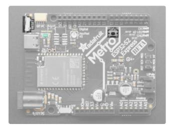
Reset button - The reset button in the top left corner is used to reset the board.
