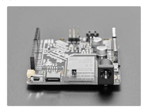
With native USB and a load of PSRAM this board is perfect for use with CircuitPython or Arduino, to add low-cost WiFi while keeping shield-compatibility.
