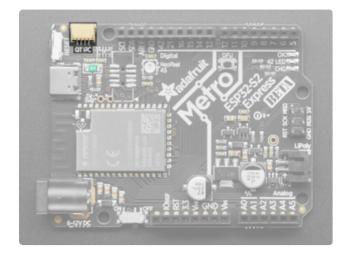
STEMMA QT () - This JST SH 4-pin connector breaks out I2C (SCL, SDA, 3.3V, GND). It allows you to connect to various breakouts and sensors with STEMMA QT connectors () or to other things using assorted associated accessories ().
